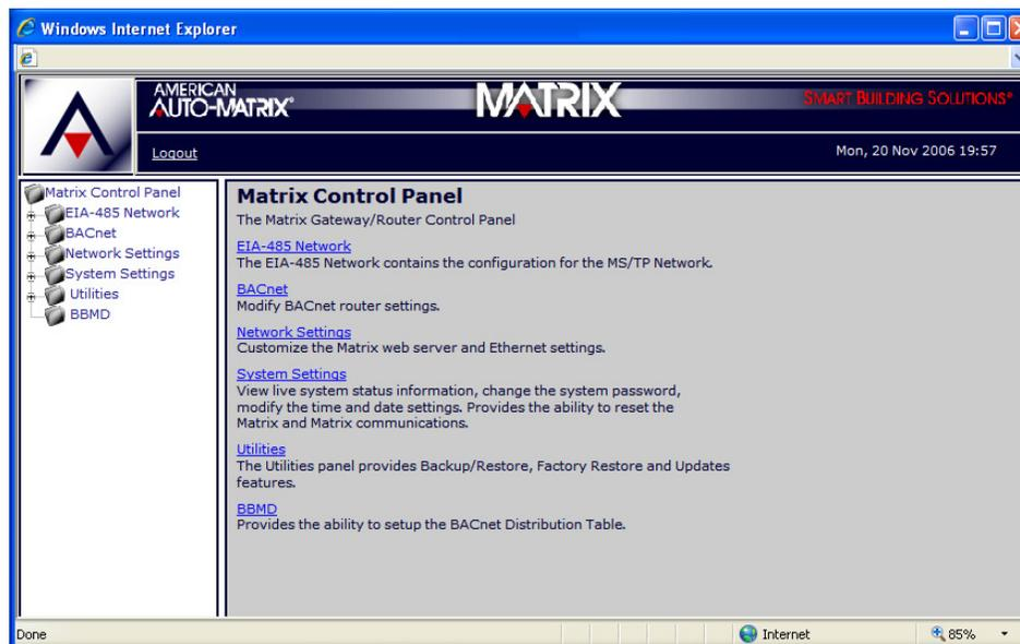
Figure 3-3 Matrix Router Control Panel and Navigation Tree
